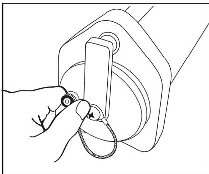
7. Small aliquots of sample water can be removed from the chamber by removing the expansion plug on the chamber end cover. Turn the thumb knob to loosen the plug. When replacing the plug, tighten the thumb knob to “finger tight”. Larger aliquots of the sample can be poured from the chamber by opening one chamber end cover.
